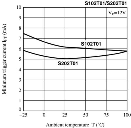
Fig.6 Minimum Trigger Current vs. Ambient Temperature (Typical Value)
