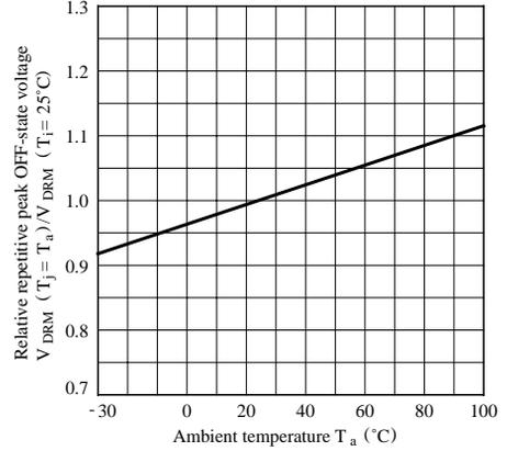
**Fig. 5-b Relative Repetitive Peak OFF-state Voltage vs. Ambient Temperature (S21MS4)**
