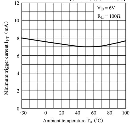
**Fig. 4-b Minimum Trigger Current vs. Ambient Temperature (S21MS4)**
