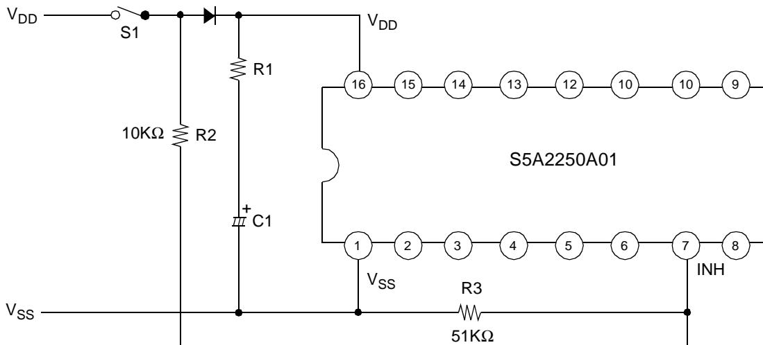
**NOTE:** If  $V_{DD} - V_{SS}$  become below 4.0V, the backup is impossible.
