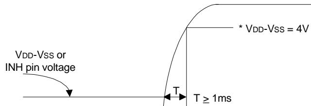
**NOTE:** If the voltage between  $V_{DD}$  and  $V_{SS}$  is below 4.0V, the auto-initializing function is actuated.
