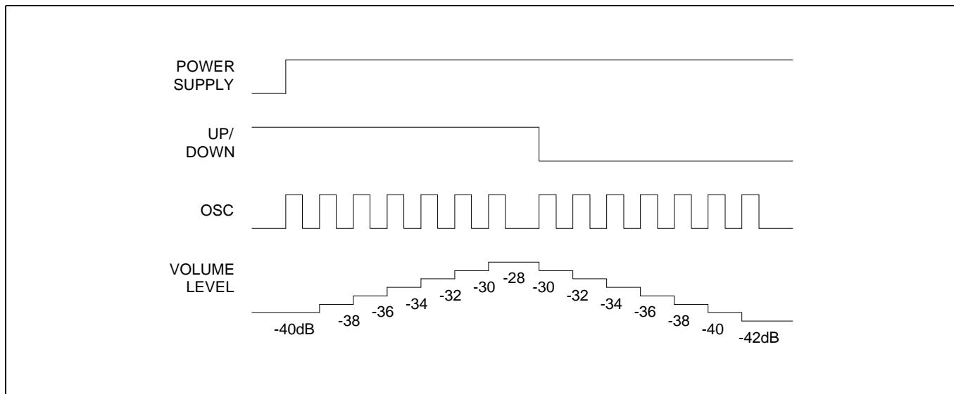
As soon as the UP key is pressed after power on, the U/P pin is placed in the up state at "H" level, and the oscillator is actuated.
