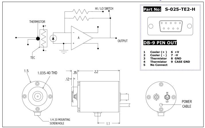
This unit is a high performance photodiode/receiver operated with a thermoelectric cooler for stabilization/cooling with a dual gain FET input transimpedence amplifier. The output voltage is proportional to the input signal current:  $\mathbf{V_{out}} = \mathbf{I_{signal}} \cdot \mathbf{R_f}$ . The PD/AMP is a DC coupled dual gain system. Care should be taken in shielding the unit from stray light during operation to prevent saturation of the amplifier (and potential failure).
