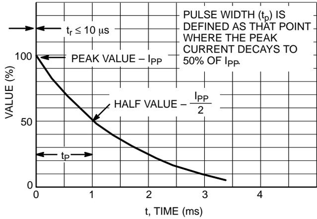
Figure 4. Pulse Waveform
