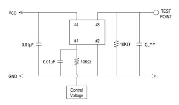
\*\*CL = 10pF (Including probe and jig capacitance)
