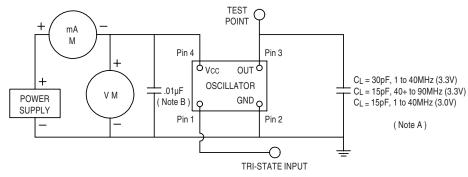
NOTE: A. CL includes probe and fixture capacitance.
