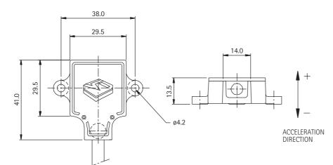
The accelerometer weighs approximately 60g with a standard 30cm PUR cable (3 x 0.5 mm<sup>2</sup>), excluding connector.
