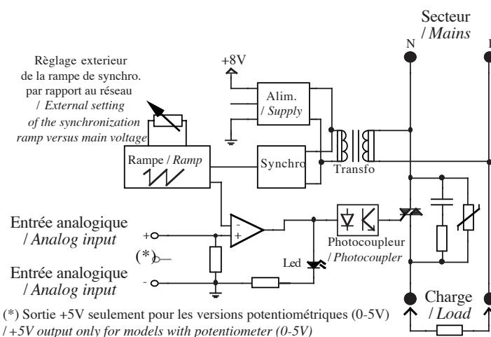
Branchements type puissance et potentiomètre / Typical potentiometer and power wiring :
