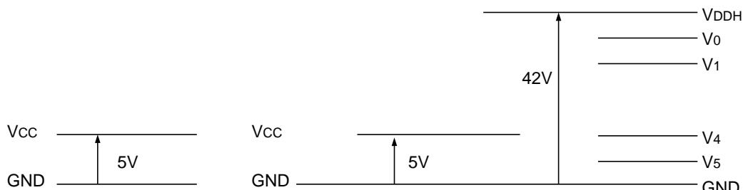
(Note 3) If the logic power is made floated or becomes  $Vcc = 2.6V$  or less while LCD drive power is being applied, the LSI may be permanently damaged and avoid these situations. Pay particular attention when determining the power supply sequence for turning on and off of the system power.
