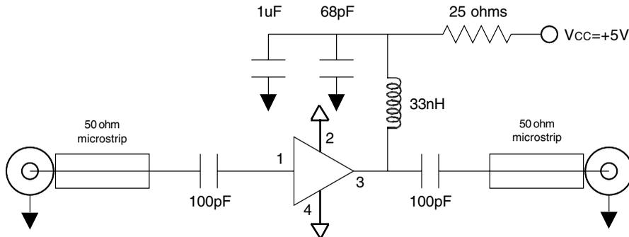
**Application Schematic for +5V Operation at 1900 MHz**
