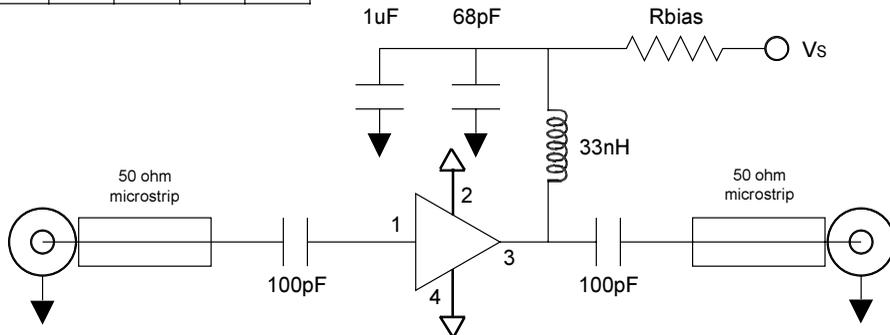
**Application Schematic for Operation at 1950 MHz**
