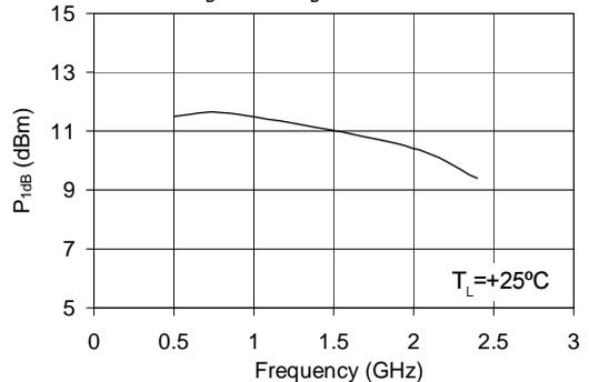
**Typical RF Performance Over Temperature ( Bias:  $V_D = 2.6$  V,  $I_D = 35$  mA (Typ.) )**
