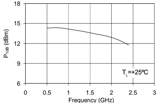
**Typical RF Performance Over Temperature ( Bias:  $V_D = 3.2$  V,  $I_D = 45$  mA (Typ.) )**
