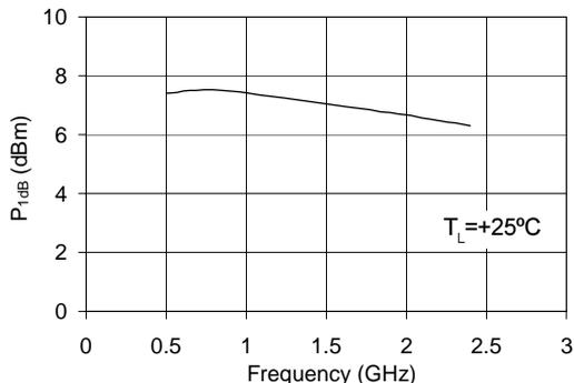
**Typical RF Performance Over Temperature ( Bias:  $V_D = 2.2$  V,  $I_D = 20$  mA (Typ.) )**
