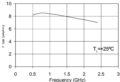
**Typical RF Performance Over Temperature ( Bias:  $V_D = 2.7$  V,  $I_D = 20$  mA (Typ.) )**
