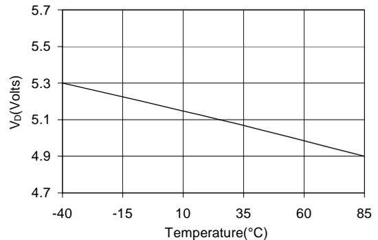
\* Note: In the applications circuit on page 4,  $R_{BIAS}$  compensates for voltage and current variation over temperature.
