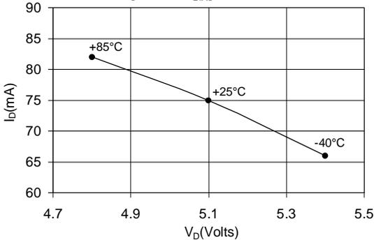
**$V_D$  vs. Temperature for Constant  $I_D = 75$  mA**
