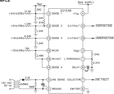
In this example, the SG1548 simultaneously monitors four DC voltages: +5V, +24V, and  $\pm15V$ . Three different fault tolerances are programmed:  $\pm5\%$  on the two 15V supplies,  $\pm10\%$  on the +5V supply, and  $\pm20\%$  on the +24V supply. The  $5\mu$ F delay capacitor provides 125 milliseconds of fault delay.
