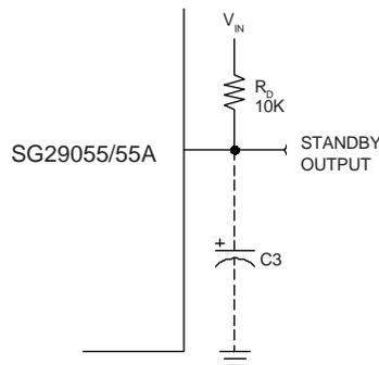
FIGURE 1. Disabling Standby Output to Eliminate C3
