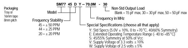
Consult factory for available frequencies and specs. Not all options available for all frequencies. A special part number may be assigned. Frequency Stability is inclusive of frequency shifts due to calibration, temperature, supply voltage, shock, vibration and load
