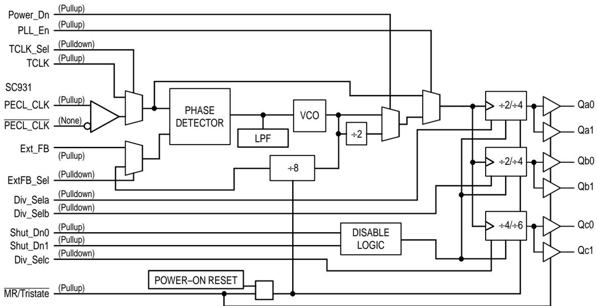
Figure 2. Logic Diagram
