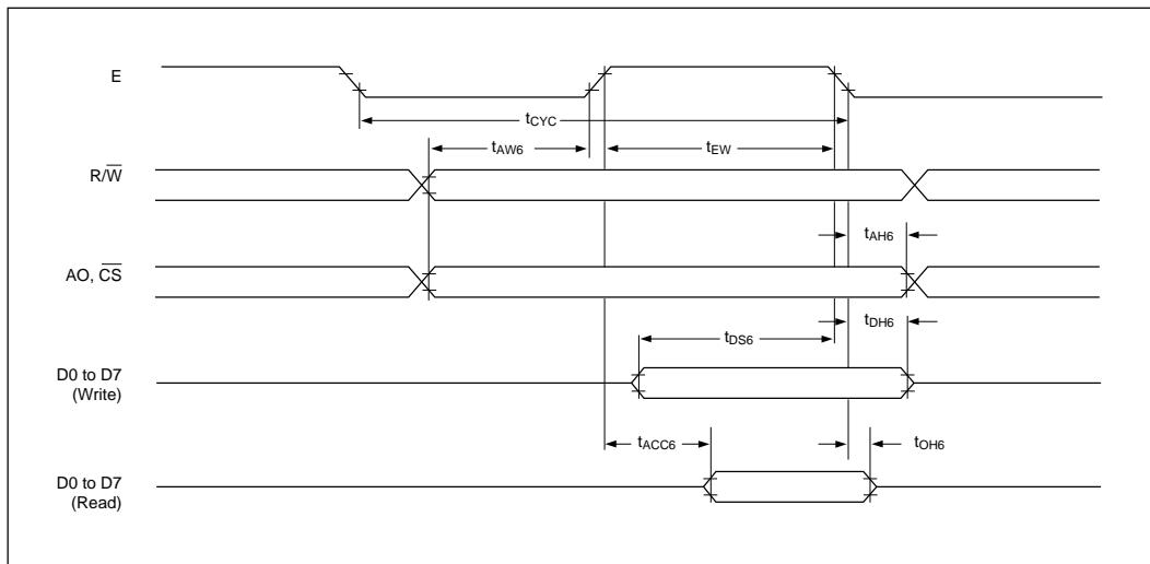
**Note:** t<sub>CYC6</sub> indicates the interval during which CS is LOW and E is HIGH.
