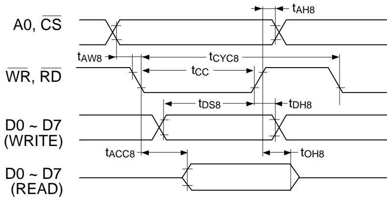
T<sub>a</sub> = -20 to 75°C, V<sub>SS</sub> = -5.0V ± 10%, Unit: ns
