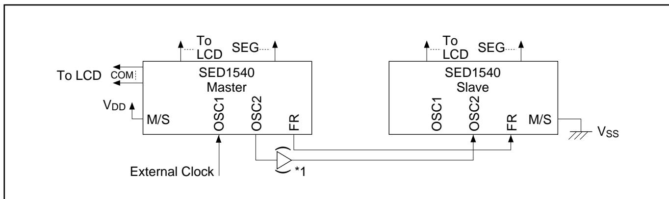
\*1. For connection to more than one slave LSI, a CMOS buffer must be used.
