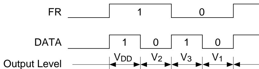
COM0– LCD common (row) driving output. (The COM2 and COM3 output state is changed by the Duty Select command. One of the VDD, V1, V2, and V3 levels is selected by a combination of the output of the common counter output and the FR signal.
