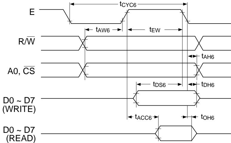
T<sub>a</sub> = -20 to 75°C, V<sub>SS</sub> = -5.0V ± 10%, Unit: ns
