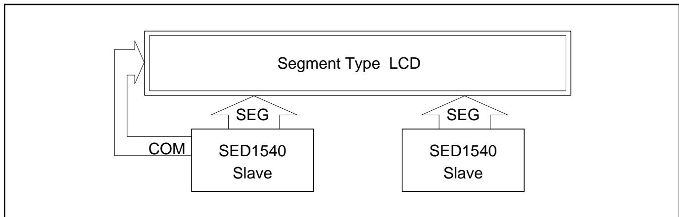
The slave IC may be omitted in this connection. The panel can be driven with the master IC alone.
