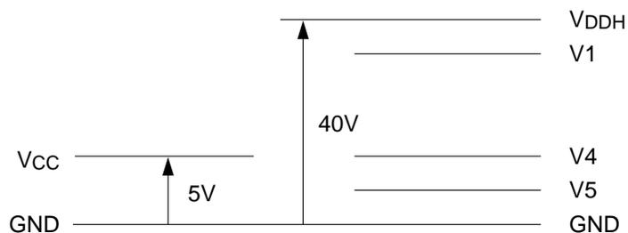
Note 2. If the logic circuit power supply comes to float while voltage is applied to the power supply of the liquid crystal driving circuit, the LSI may be broken permanently. So, prevent the logic circuit power supply from floating. Pay special attention to the power supply sequence when the system is switched on or off.
