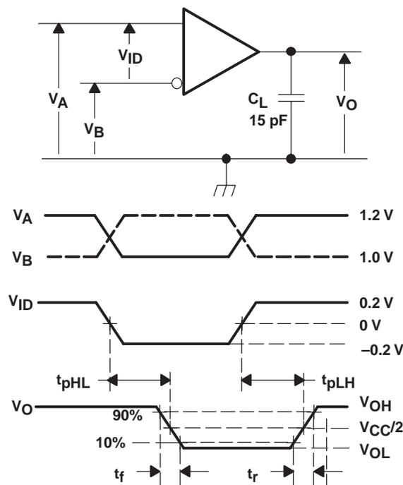
NOTES: A. All input pulses are supplied by a generator having the following characteristics:  $t_r$  or  $t_f \leq 1 \text{ ns}$ , frequency = 50 MHz, duty cycle =  $50 \pm 5\%$ .  $C_L$  is a combination of a 20%-tolerance, low-loss ceramic, surface-mount capacitor and fixture capacitance within 2 cm of the D.U.T.
