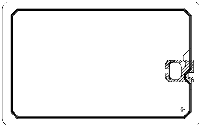
Module combined with antenna on foil (inlay)
