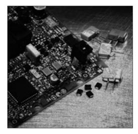
Tyco Electronics SiBar® thyristor surge protectors are designed to protect sensitive telecommunications equipment from the hazards caused by lightning, power contact, and power induction. These devices have high surge capability to protect against transient faults and high off-state impedance, rendering them transparent during normal system operation.
