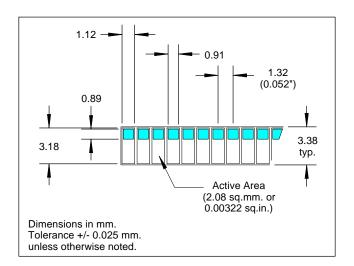
To order this part the 'XX' refers to the number of elements in the array (from 02 to 16 elements).
