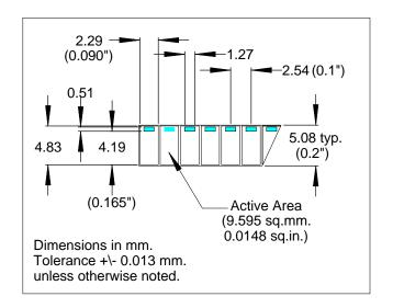
To order this part the 'XX' refers to the number of elements in the array (from 02 to 08 elements).
