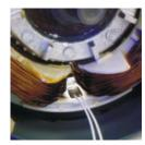
The Thermal-Tab RTD represents a major advance in the technology of temperature sensing. It features a highly accurate and stable platinum thin-film element mounted onto a flexible substrate, connected via Teflon-insulated leads, and sealed with an elastomeric coating. The result is a sensor with unprecedented economy and ease of use.
