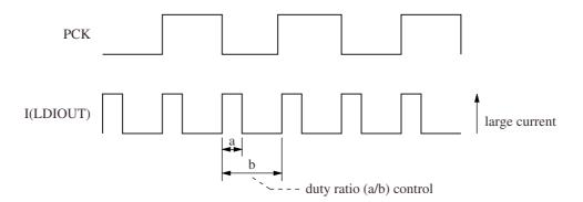
The output pulse current (LD chopper signal) on LDIOUT is automatically adjusted to maintain roughly constant duty ratio, even for changes in frequency. The LD chopper signal duty ratio can be adjusted by changing the resistance  $R_{DUTY}$  connected between the DUTYADJ and GND pins, as given by the following equation.
