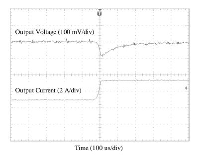
Typical transient response to step decrease in load from 50% to 25% of full load at 0.1A/µs slew rate and 48V input.
