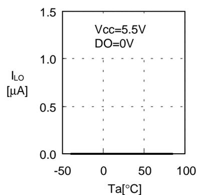
1.15 Output leakage current  $I_{LO}$  – Ambient temperature  $T_a$
