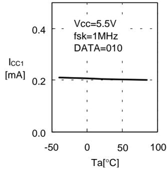
1.2 Current consumption (READ)  $I_{CC1}$  – Ambient temperature  $T_a$
