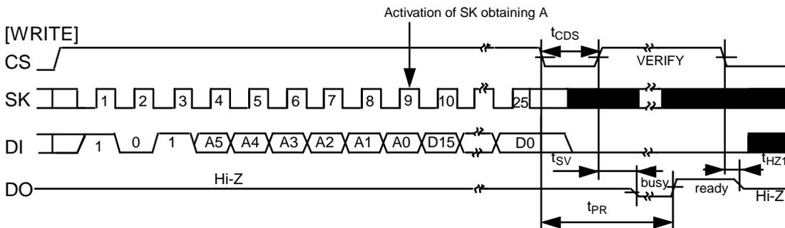
Case in which, during a command entry, CS is changed from H to L with a timing that differs by a predetermined minimum number of clocks.
