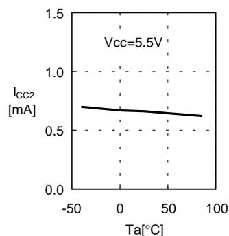
1.8 Current consumption (PROGRAM)  $I_{CC2}$  – Ambient temperature  $T_a$
