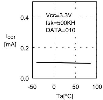
1.3 Current consumption (READ)  $I_{CC1}$  – Ambient temperature  $T_a$
