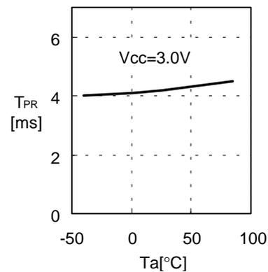
2.5 Program time  $T_{PR}$  – Ambient temperature  $T_a$
