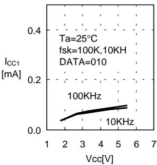
1.6 Current consumption (READ)  $I_{CC1}$  – Clock frequency  $f_{SK}$
