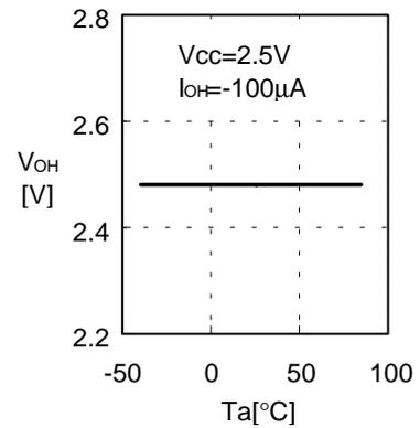
1.19 High level output voltage  $V_{OH}$  – Ambient temperature  $T_a$
