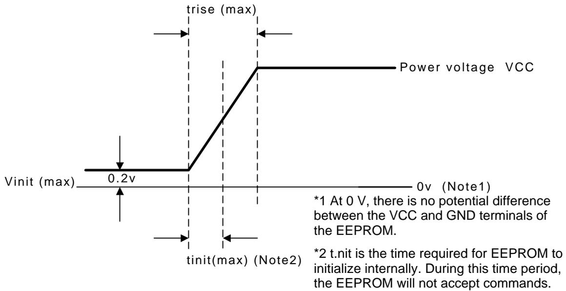
Fig. 1 Activation of the Power Voltage
