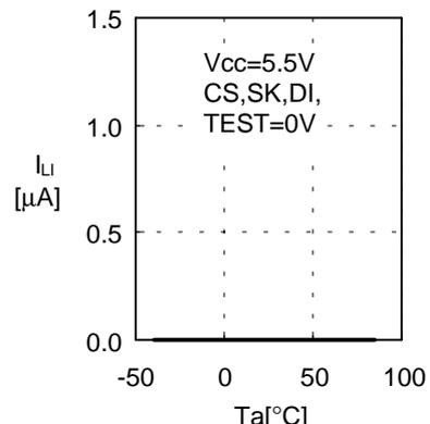
1.13 Input leakage current  $I_{LI}$  – Ambient temperature  $T_a$
