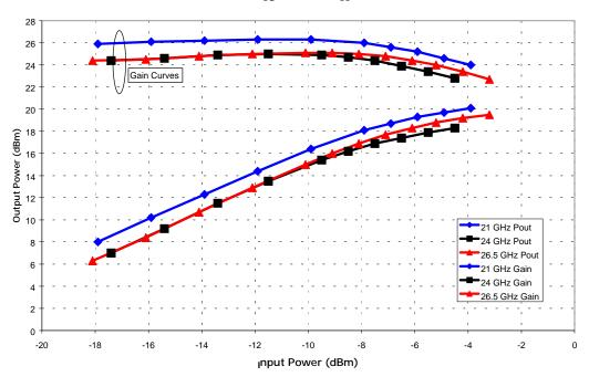
RMWL24001 Driver Amplfier Typical WideBand S-Parameters. Measurements Include 50 Ohm Test Fixture.  $I_{DQ} = 240 \text{ mA V}_{DD} = 4 \text{ V}$
