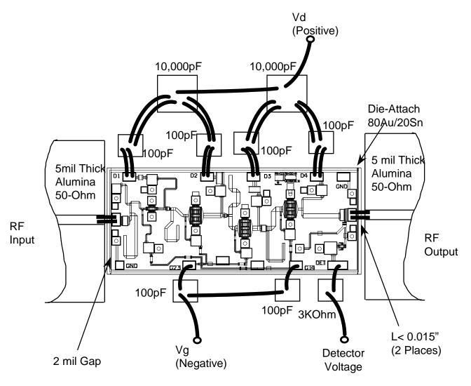
Note: Use 0.003" by 0.0005" Gold Ribbon for bonding. RF input and output bonds should be less than 0.015" long with stress relief.
