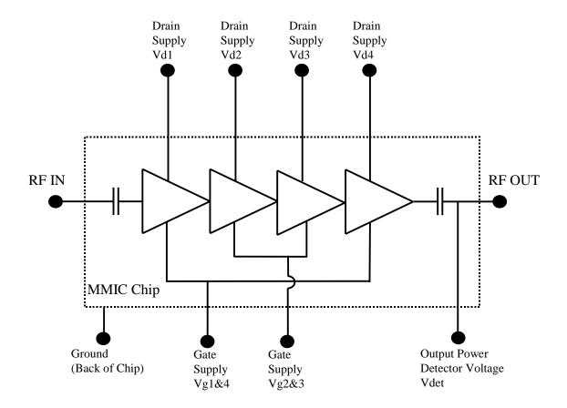
Note: Detector delivers 0.1 V DC into 3k  $\Omega$  load resistor for >+7 dBm output power. If output power level detection is not desired, do not make connection to detector bond pad.
