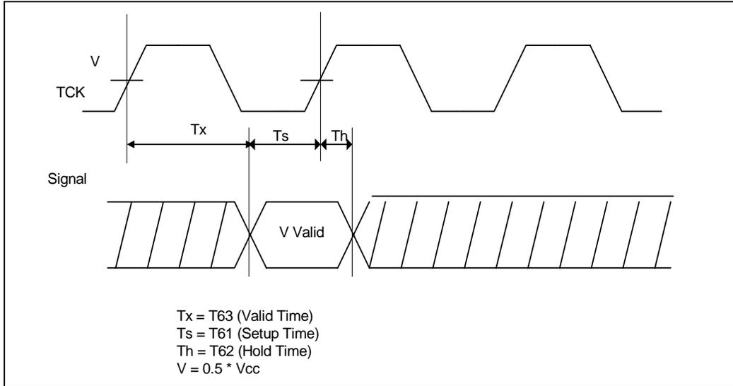
**Figure 22. ITPCLKOUT Valid Delay Timing**
