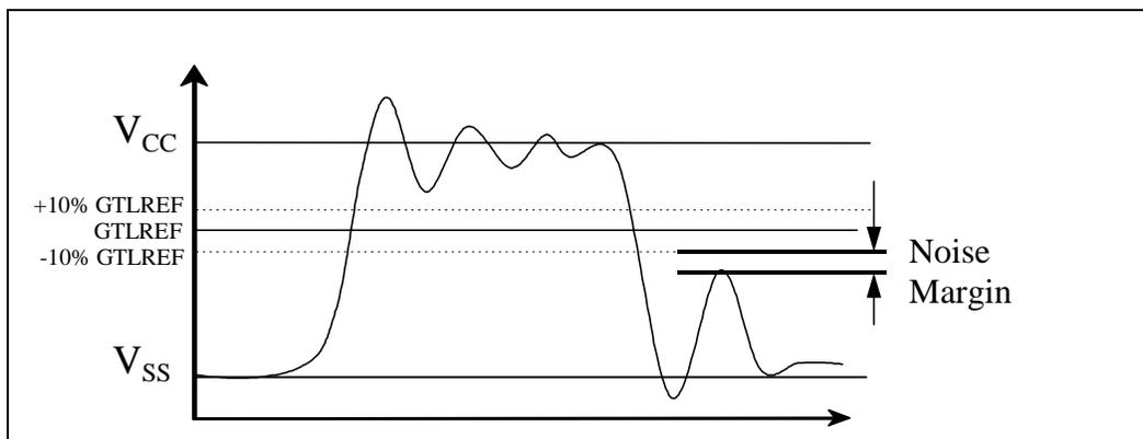
**Figure 28. Low-to-High System Bus Receiver Ringback Tolerance for PWRGOOD and TAP Buffers**
