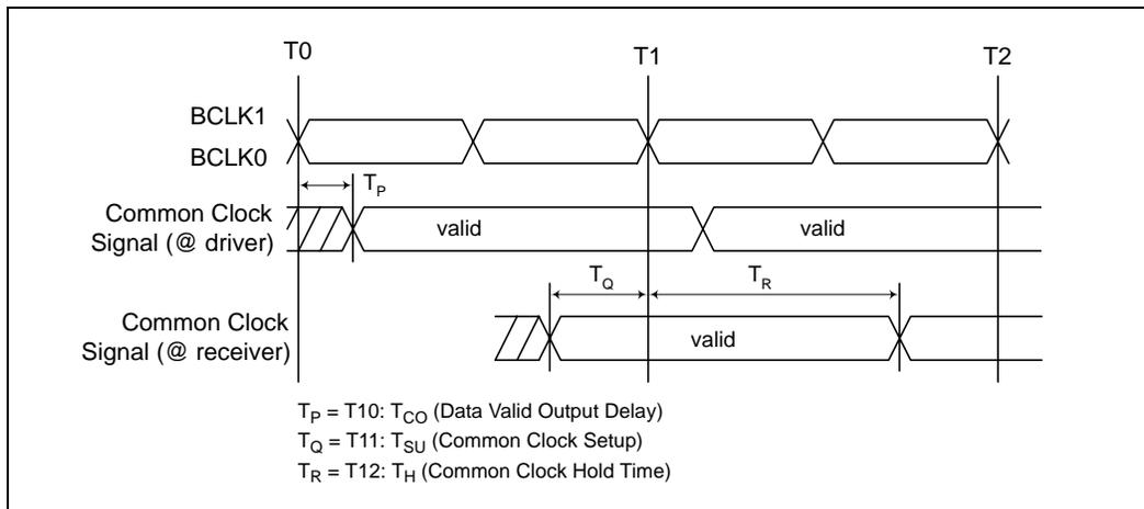
**Figure 13. System Bus Reset and Configuration Timings**
