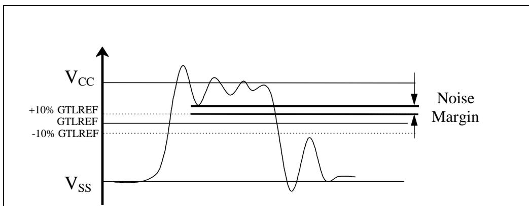
**Figure 27. High-to-Low System Bus Receiver Ringback Tolerance**
