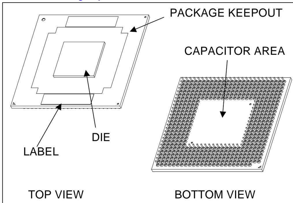
Figure 32. Micro-FCPGA Package Top and Side View
