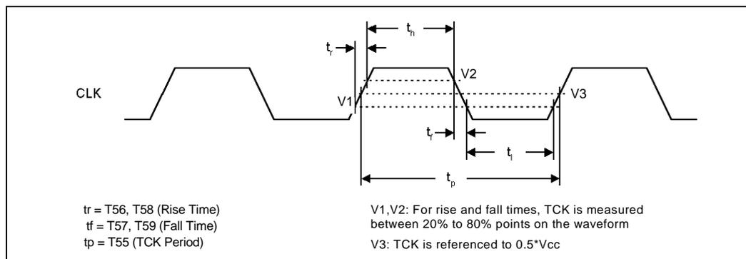
Figure 10. Differential Clock Waveform
