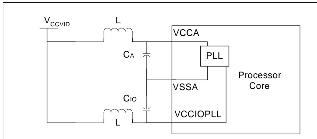
**Figure 3. Phase Lock Loop (PLL) Filter Requirements**
