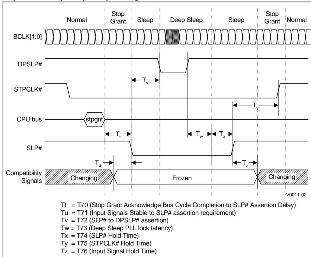
**Figure 24. Enhanced Intel SpeedStep Technology/Deep Sleep Timing**
