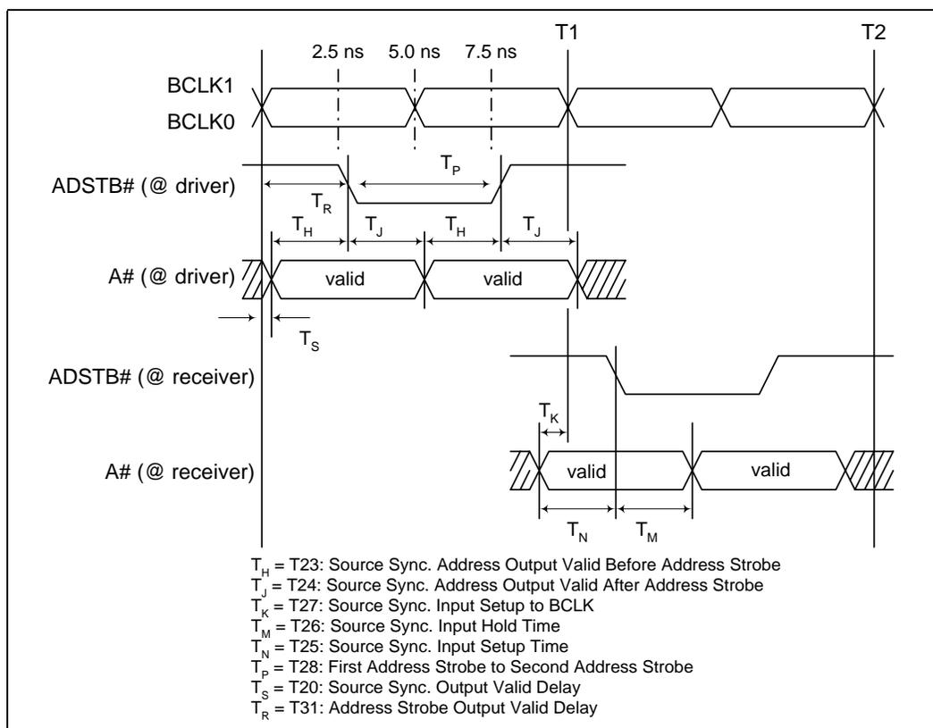
Figure 15. Source Synchronous 4X Timings
