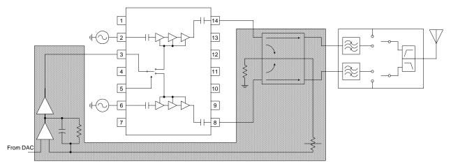
\*Shaded area eliminated with Indirect Closed Loop using RF3110
