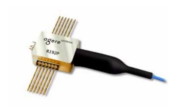
Featuring improved sensitivity for optimum performance in noisy, amplified systems, the R192P Receiver is manufactured in a compact, 16-pin surface-mount package (above), and is also available with a convenient mounting bracket (below).
