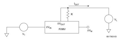
2. CMRR is measured with  $V_1 = +15V/-5V$ ; R is RA, RB, RC or RD;  $I_{OUT} = constant$ . This parameter is to define the current measurement error due to the input voltage  $V_1$ . It guarantees all ranges and  $\pm$  full scale  $I_{OUT}$ .
