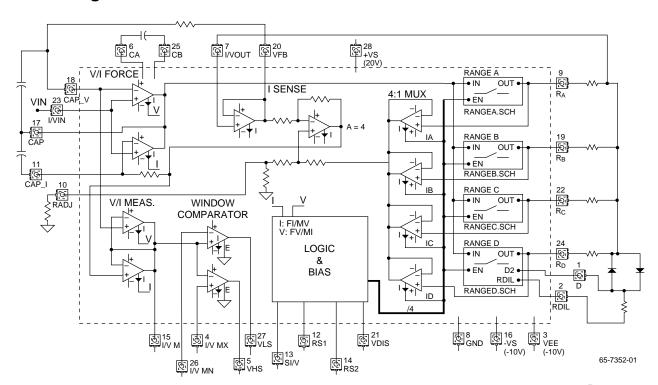
I/VIN pin (please refer to block diagram). The I/VM pin provides a voltage proportional to the DUT current.  $V(I/VM) = (4~x~R~x~I(DUT)), \mbox{ where } R \mbox{ is the external range resistor } (0.05\% \mbox{ tolerance}) \mbox{ and } I(DUT) \mbox{ is the current supplied to the load. The resistors in the application circuit were chosen using this formula R range = (2V/Imax), for Range A this is <math display="inline">RA = 2/20~\mu A$  or 100K.
