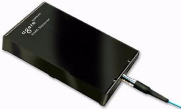
Manufactured in a low-profile, 24-pin package, the R480-Type receiver features either an avalanche or PIN photodetector, a transimpedance amplifier, and a limiting amplifier IC.
