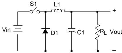
Figure 2. Simple Buck DC-DC Converter
