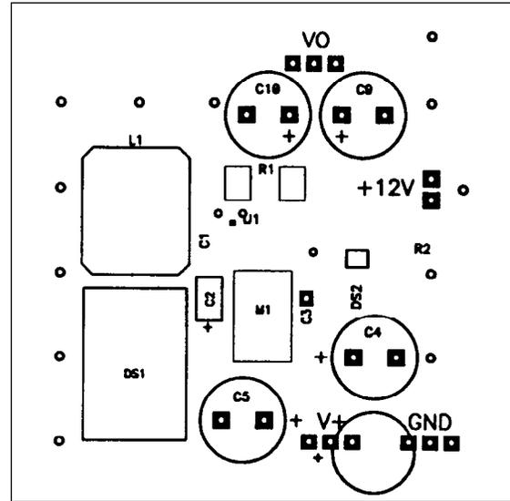
Figure 3. Sample PCB Layout for RC5601
