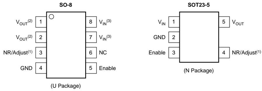
NOTE: (1) For REG101A-A: voltage setting resistor pin. All other models: noise reduction capacitor pin.
