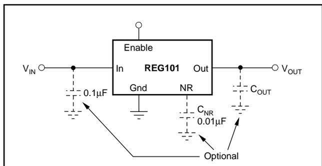
FIGURE 1. Fixed Voltage Nominal Circuit for REG101.
