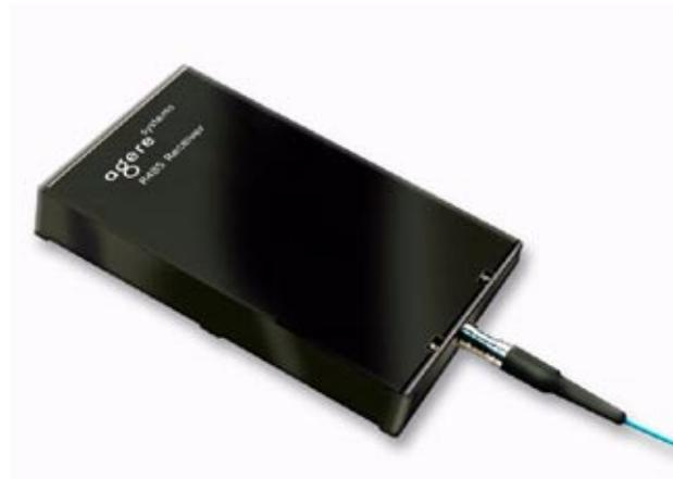
Manufactured in a low-profile, 24-pin package, the R485-Type Receiver features either an avalanche or PIN photodetector, a transimpedance amplifier, a limiting amplifier, and a clock and data recovery IC.
