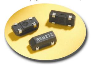
Quartz crystals ordinarily generate much higher frequencies. In order to generate the standard 32.768 KHz for convenient divide-by-60 countdowns, Raltron has shaped the internal crystal into a little tuning fork. This new tuning-fork crystal is hermetically sealed in an SMT package and designated Model RSM-200
