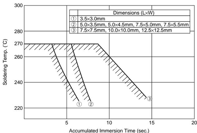
Perform soldering within tolerance range (shaded portion).
