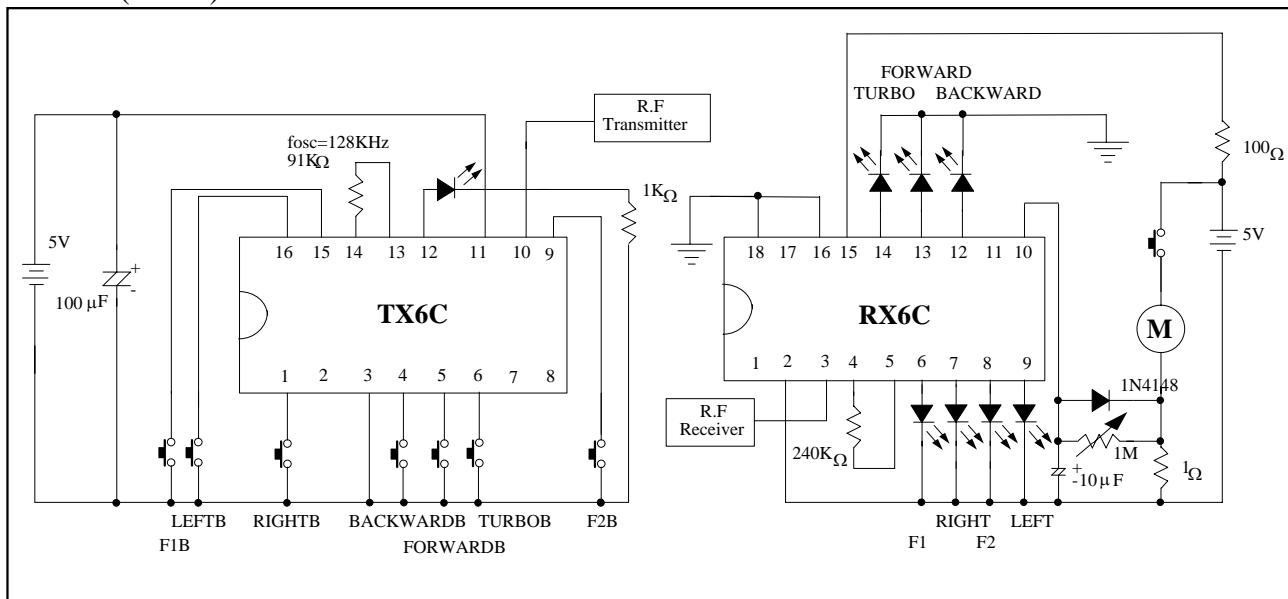
TX6C output pin (SO) has an inverted phase with RX6C input (SI). If TX6C & RX6C are connected without using a RF module, an inverter has to be inserted between this 2 pins.
