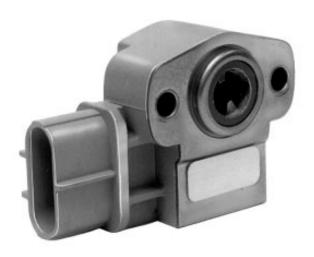
RP Series rotary position sensor is intended for angular position sensing applications where freedom from wear-out failure mechanisms is important. A patented, symmetrical magnetic circuit is used to generate a linear magnetic field as a function of rotor angle. This linear magnetic field is converted to a linear DC voltage by a highly precise Hall effect integrated circuit. The symmetrical magnetic circuit minimizes errors due to rotor runout and assembly tolerances.
