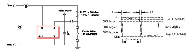
\*CL (Capacitive Load): Includes the input capacitance of oscilloscope.
