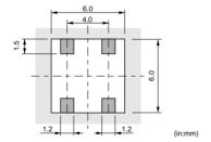
The solder resist should be printed except for the land
