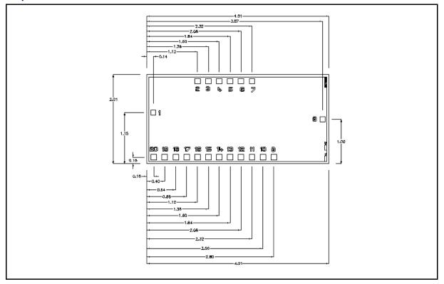
Die size:  $4.01 \times 2.01 \text{mm}$  RF bond pads (1 & 8):  $120 \times 120 \mu \text{m}$  All other bond pads:  $120 \mu \text{m} \times 120 \mu \text{m}$
