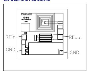
Die size: 1.22 x 1.22mm Bond pad size: 120µm square Die thickness: 200µm
