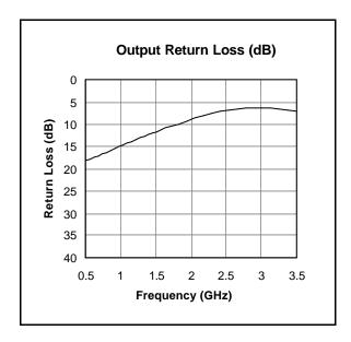
Note:- Two SMA connectors and bondwires are included in the above data.
